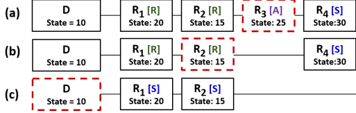
Figure 8. Inferring the current device status. The dashed boxes point to the current device status in three different scenarios.
